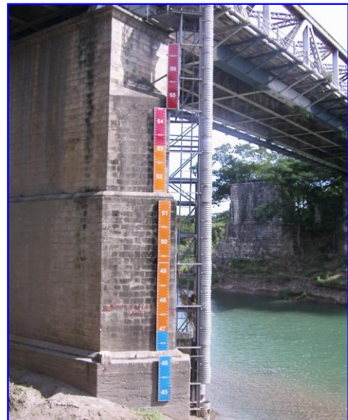
Plate 1: Flood Gauge at May Pen Railway Bridge (part of Rio Minho Flood Warning System)
