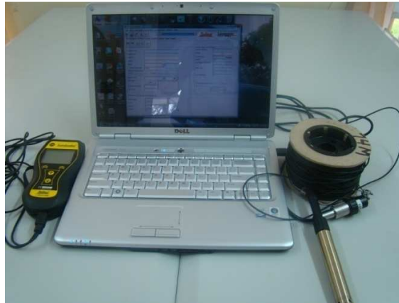
Figure 2: Solinst lever loader logger (right) with hand held device (left) and laptop for data retrieval/storage (centre)
