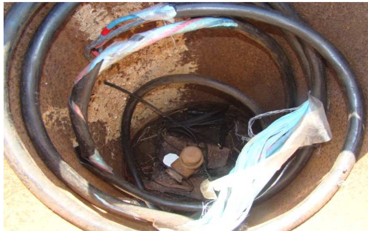
Figure 1: Solinst lever loader logger in well for continuous pump testing
