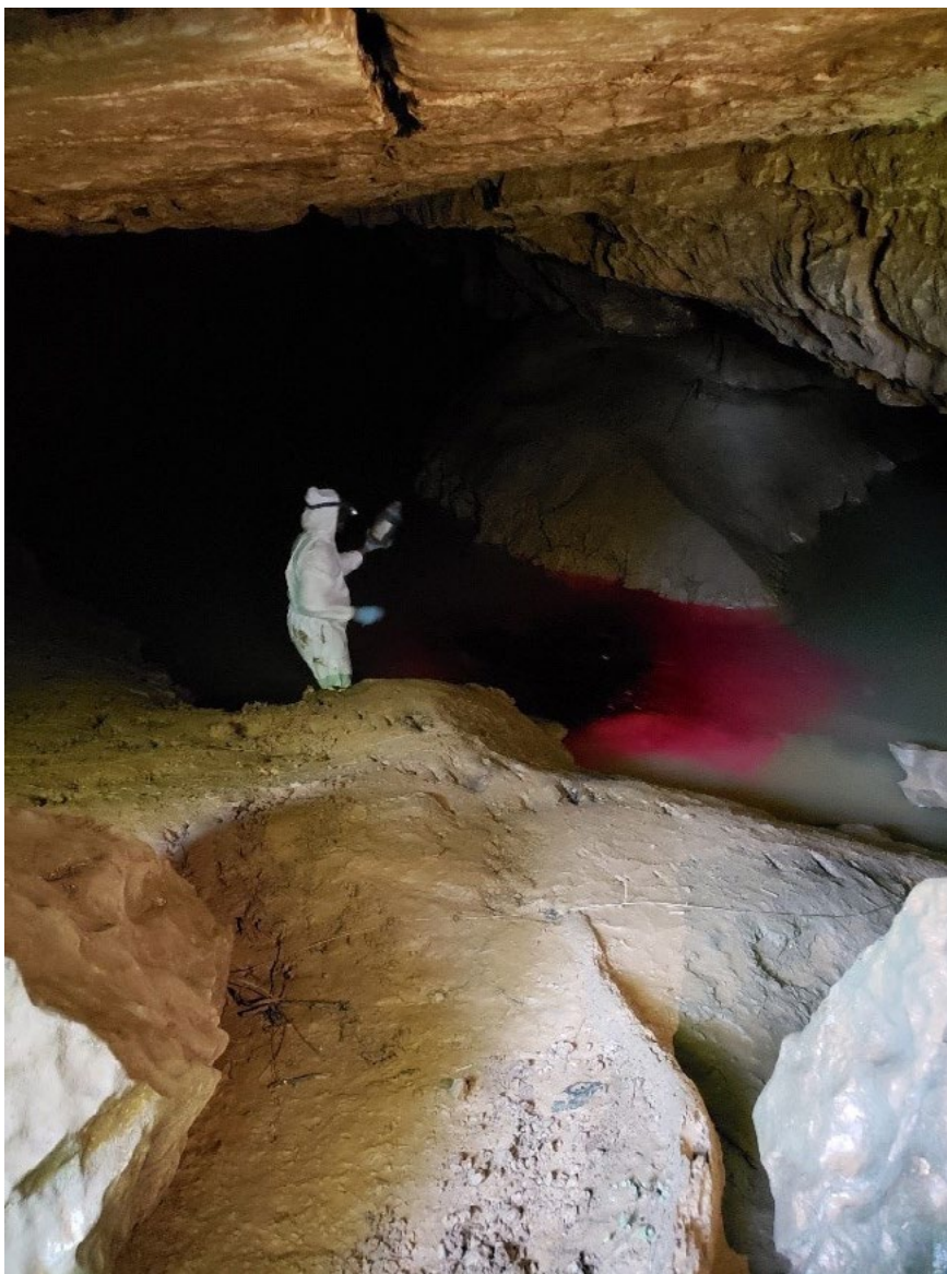
Figure 16: Dye Injection at Blue River Sink (featuring Maurice Wallace, Hydrogeologist)
