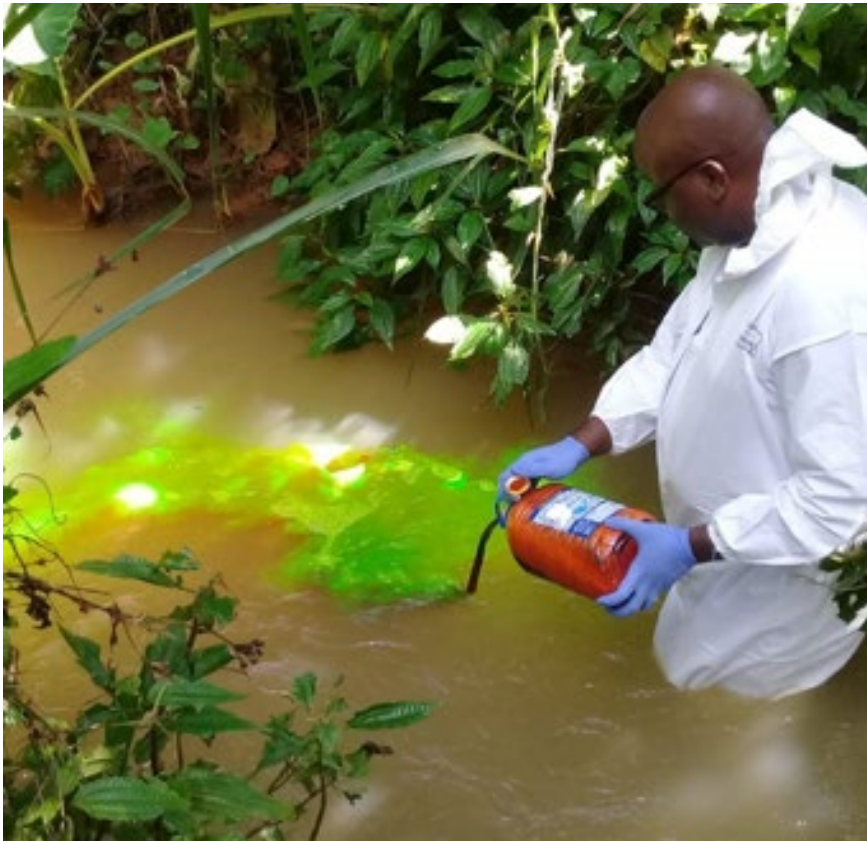
Figure 17: Dye Injection at Bottom River Sink (featuring Geoffrey Marshall, Chief Hydrologist)
